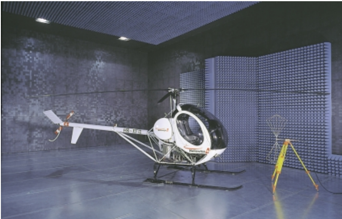
Measurement in our anechoic chamber 15,5x10x7 m (ferrites)
