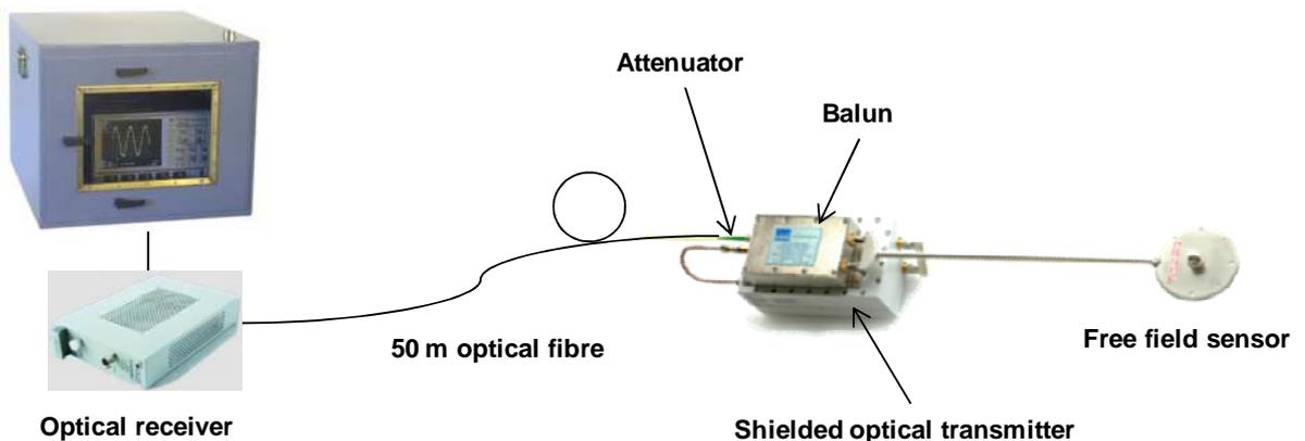
Figure 9 : free field sensor setup
