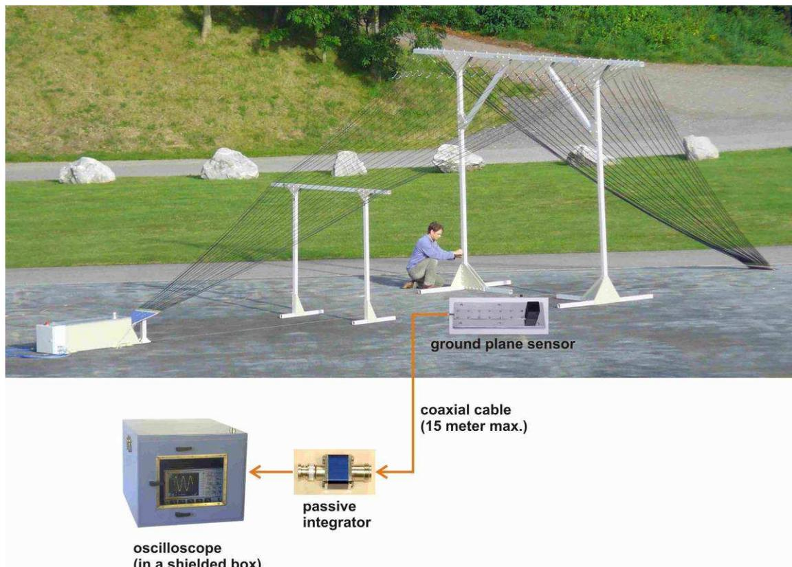
Figure 8 : Ground plane field sensor setup
