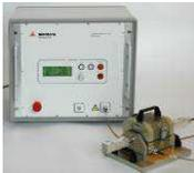
Damped Sinusoidal pulse generator
