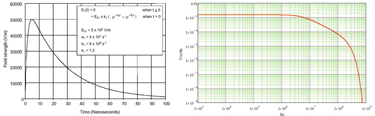
Figure 2 : MIL-STD-461E&F RS105 pulse shape and spectrum
