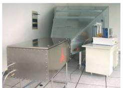
NEMP test system according to MIL STD 461E - RS105 Loading voltage 75 kV rise time 2.3 ns / duration 23 ns connected to a GTEM, 1m septum height
