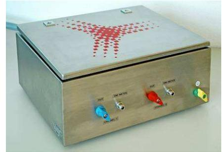
The LISN - TPD100 fulfils the MIL-STD 461 D,E and F requirements. Is consists of LISN 100 A / 270 Vac 50/60 Hz with a TPD (terminal protection device) of 100 A integrated inside the LISN and with a 20 meter shielded cable 3 x 100 A.
