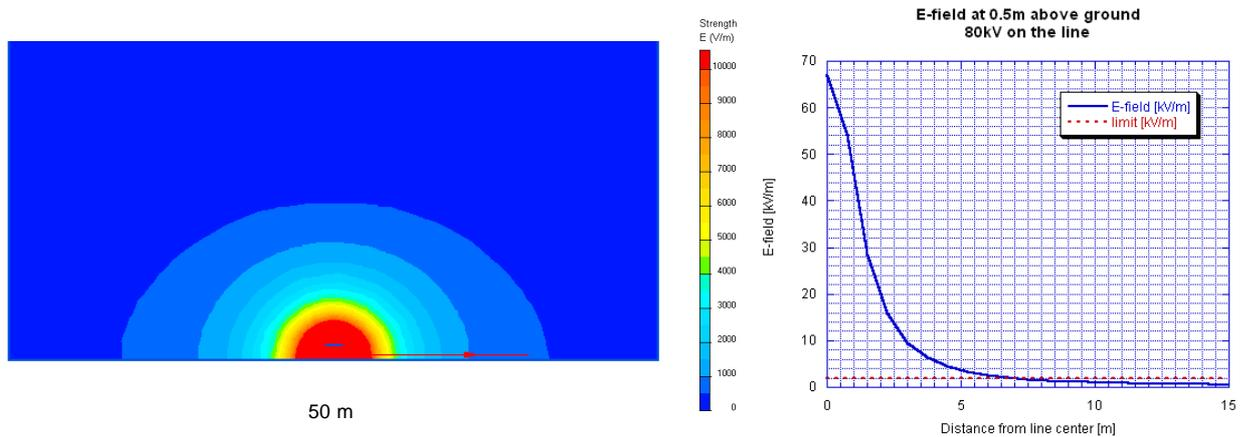
Figure 10 : electromagnetic emissions
