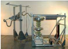
ESD 300kV and P-static test system for helicopter and airborne systems
