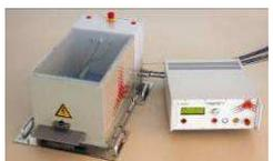
High voltage pulse generator 80kV, rise time 5 ns / duration 500 ns for Pulse Current Injection (PCI) test according to MIL STD 188/125, appendix B (short pulse)
