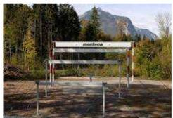
NEMP test radiation for tests according to MIL STD 461E - RS105 Marx pulse generator 800 kV, rise time 2.3 ns / duration 23 ns with 9 m high radiation line
