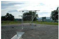
NEMP test system according to MIL STD 461E - RS105 Marx pulse generator 230 kV, rise time 2.3 ns / duration 23 ns with 3.6 m high radiation line
