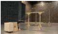
Indoor NEMP test system according to MIL STD 461E - RS105 Marx pulse generator 120 kV, rise time 2.3 ns / duration 23 ns with 2.7 m high radiation line
