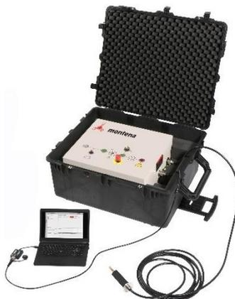
The generator is compact, battery powered for easy deployment at customer site, where power is not always available. The power autonomy is up to one day and it can be charged from a 110V – 240V power plug directly.
