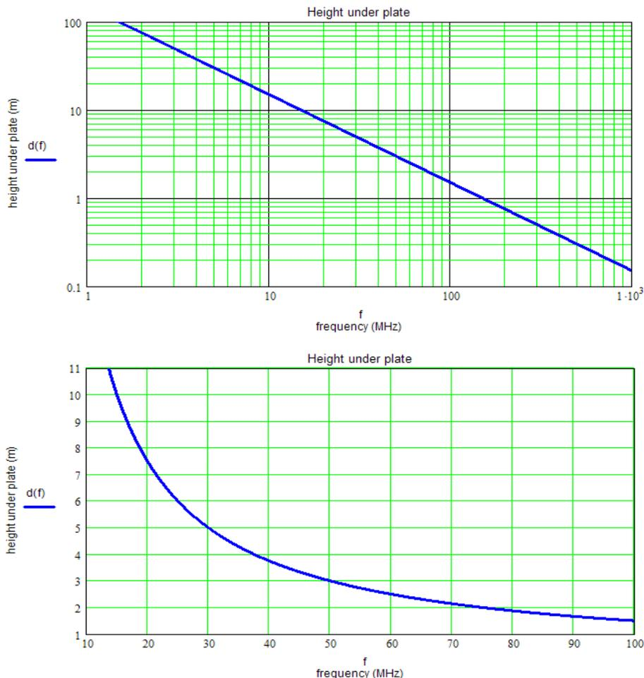
**Remark:** the devices under test placed inside the cell can produce field distortions and other modes than TEM. Therefore its dimensions have to be limited. Depending on the standard used, the height of the EUT must not exceed  $\frac{1}{2}$  or  $\frac{1}{3}$  of the height under plate. The EUT must not be too large in order to stay in the homogeneous zone inside the TEM cell or the stripline.
