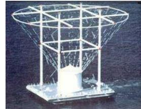
*Example of radiating simulator (conical)*
