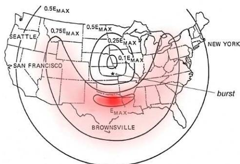
*Amplitude of the electromagnetic field on the Earth*
